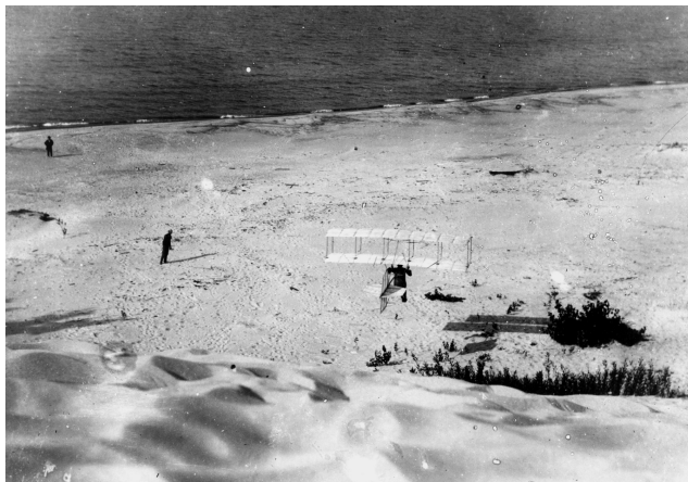
Fig. 15 Chanute-type biplane glider, September 1897. From National Air and Space Museum (NASM negative no. 7A-09329).
