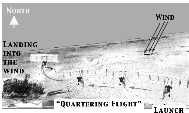
Fig. 16 “Quartering Flights,” along the sand dunes of Lake Michigan, or flying at an angle with the wind in order to remain in the ascending current over the slope to sustain flight. The machine faces north, but advances west of northwest in a wind coming from the northeast. After coming to an obstacle (a tree), the glider turns into the wind and glides away from the dune to land on the beach.
